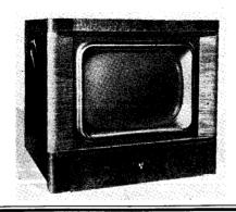
THE receiver is a superhet operating on lower sideband of vision carrier. Vision interference and sound noise suppression circuits are fitted, the former being provided with a plug and socket adjustment giving three degrees of limiting. EHT is obtained from rectified line flyback pulses. Mains consumption is approximately 120W. The receiver is assembled on two chassis with
