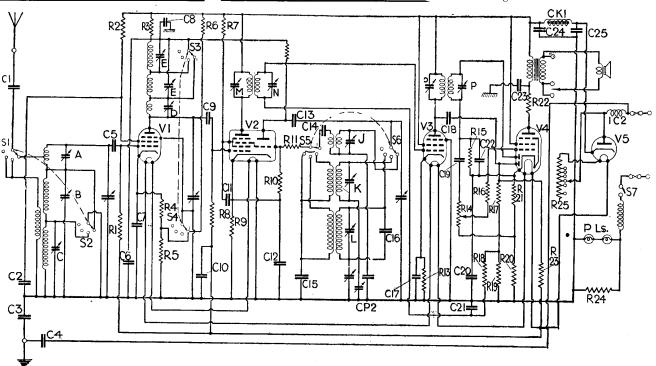
A straightforward superhet circuit is used in the Ultra 49. A radio frequency amplifier precedes the triode-hexode frequency changer. As a combined diode and output valve is employed, the set actually corresponds to many "sixes."
