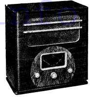
Four valves and a rectifier are used in the Ultra 49 superhet for A.C. or D.C. mains. The receiver covers three wavebands, the short section extending from 16.8 to 50 metres.
