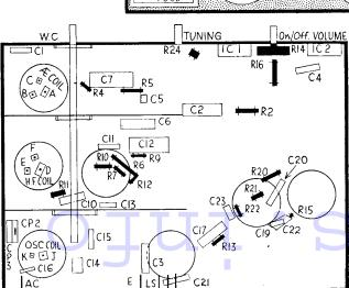
With the aid of this diagram components under the chassis can be identified easily. All resistors are in solid black, and condensers in outline. Trimmers are accessible at the bases of the coil cans.
