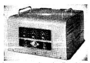
Multi purpose six-valve push-pull amplifier with 30 watts output. Input sockets provide for radio, pickup, and microphone with facilities for mixing inputs. Output sockets for high and low impedance PM speakers. Housed in crackle finished metal cabinet with lifting handles. Suitable for 200 to 250V, 40-100c/s. Made by The Trix Electrical Co., Ltd., 1-5 Maple Place, Tottenham Court Road, London, W1.
