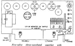
sockets for aerial, earth, high-resistance magnetic or crystal pickup and low-impedance extension speaker. Brown moulded cabinet. Suitable for 110—120, 210—250V 40—100c/s. Manufactured by R. M. Electric, Ltd., Team Valley, Gateshead 11.
