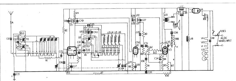
Pre-set condensers in the aerial circuit and permeability coils in the oscillator circuit provide the push-button staticals. L18 is the speaker field coil and L19 is a low-resistance series smoothing choke.
