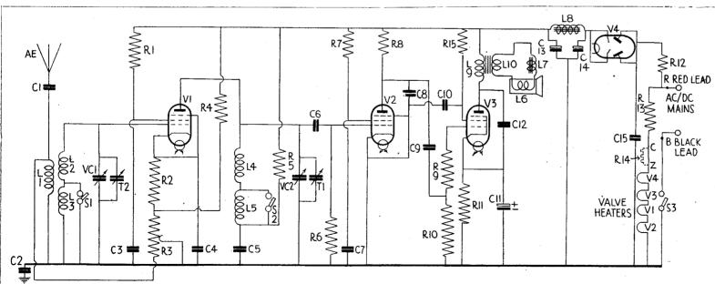
The Mite is a "straight," tuned radio-frequency three-valve, plus rectifier, portable for operation from either AC or DC mains. Volume is controlled by the bias of V1 and there is no reaction from the pentode detector valve. It should be noted that HT is applied across the second section of the tuning gang.
