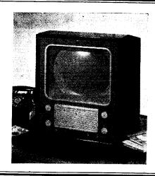
THE receiver employs a superheterodyne circuit, operating on lower sideband of vision carrier, in which the RF and frequency-changer stages are common to vision and sound channels. Vision interference and sound noise suppression circuits are incorporated and EHT is obtained from line flyback. Channel selection is by plugging in an appropriate set of aerial, RF and oscillator coils and retuning oscillator trimmer.
