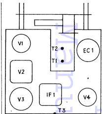
How components are arranged on the top of the chassis. It is a single waveband set with only three trimmers.
