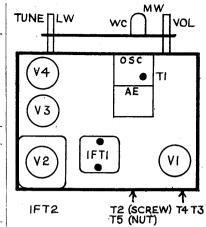
Above, the top of chassis layout. In the circuit below the alternative switch connections shown are those used when part number 339-5003 is employed instead of the standard 33-5213.
