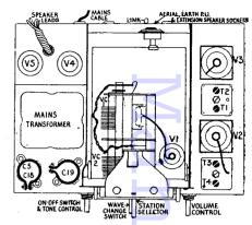
The top-of-chassis layout diagram of the Philco receiver, indicating valve and some trimmer positions. location of the remaining trimmers is below deck, and they are grouped above the wavechange switchbanks as shown in the diagram on the left.
