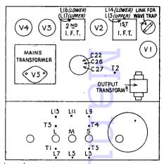
The chassis of the AC model, showing trimmer positions. The same diagram applies to the DC version as regards trimming and general layout.
