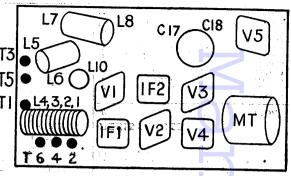
Tune and inject 20 m. (15 mc.) and VALVE READINGS adjust loop of L1 while rocking gang. Tune and inject 30 m. (10 mc.) and adjust shape of trimming loop of L5.
