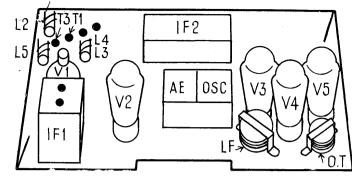
This set is a compact model and the chassis a little unusual. Two trimmers and the adjustable coil cores are located as shown. Two others are on the aerial frame.
