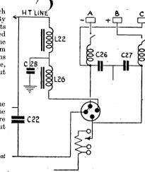
Models 505 and 280 RGs incorporate a plug and socket for conversion to AC by means of a metal rectifier unit. Models 404 and 278 have two PLs and no L26, C28.
