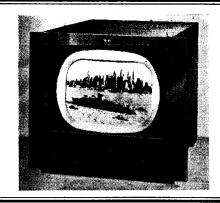
THE receiver is a superhet designed to operate on lower sideband of vision carrier. The RF and frequency-changer stages are common to vision and sound channels. A separate temperature-compensated local oscillator is employed. Vision interference and sound noise suppression circuits are incorporated; EHT is obtained from line flyback pulses. Mains consumption is approximately 130W.
