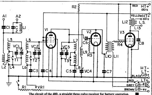
An extension speaker can be used with the internal speaker by connecting the extension leads to the LS section of the gang. Positive feedback from the terminals: these leads should go direct to a 2-ohm speech coil of the external speaker.
