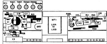
to grid V3; HT removed from V1; output 2 socket brought into circuit for monitoring or connection to external amplifier; V2A cathode capacitor C9 taken out of circuit.
