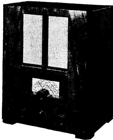
The T.R.F.3 battery set by G.E.C. is a "straight three" which includes a number of refinements which ensure a high performance over both wavebands and ease of control.
