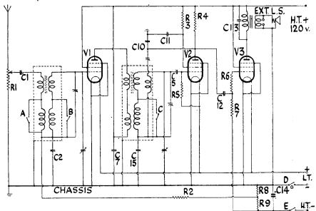
Iron-core aerial transformer and H.F. coils are employed in the Battery S.P. Three. The volume control is in the aerial circuit, and a feature is the provision of pre-set information reaction ember
