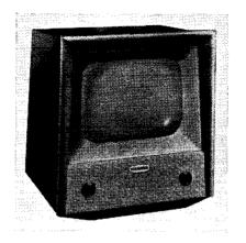
THESE receivers differ only in CRT size and type of cabinet. Both the 992T and 994T employ a Mullard CRT, type MW36-24 (14in. rectangular) and are table and console models respectively. Table model 996T incorporates a Mullard MW43-64 tube (17in. rectangular), which requires a slightly weaker focusing magnet and has an additional electrode externally connected to cathode. Both types of tube have dark glass screens. All models employ a tinted filter.
