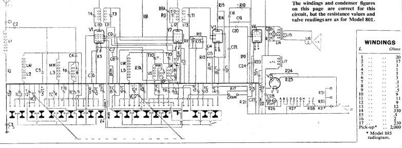
condensers across the aerial and oscillator coils as required. The aerial trimmers are TC1-TC7 in the accompanying circuit diagram and the oscillator trimmers TC8-TC14. The setting up of the station button trimmers is as described in the reviews of the Models 881 and 884. **GANGING**
