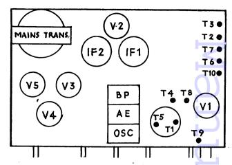
The top of the chassis is arranged in a logical manner with all the trimmers accessible from above.
