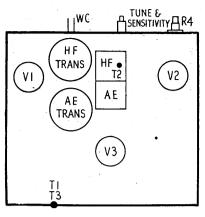
A simple battery three with reaction, the B39 presents few service problems. Aerial and H.F. circuits can be aligned.
