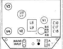
This diagram identifies the main features on the chassis of the Ekco AD65. The parts indicated are grouped round the loudspeaker. Most of the trimmers are associated with the gang condenser.
