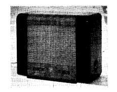
Five-valve superhet giving four preset switch-selected stations. Fitted with internal frame aerial, sockets for external aerial and earth, a low-impedance extension speaker and a high-impedance magnetic or crystal pickup. Housed in walnut veneered table type cabinet. Suitable for use on 200-250V, 50-100c/s mains. Made by E. K. Cole Ltd., Southend-on-Sea. Essex.
