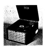
An electric record reproducer for operation from AC mains supplies 200-250V, 50 cycles. Consists of a two-stage amplifier, with negative feedback, feeding into a 61-inch permanent magnet loudspeaker. The pick-up is a Decca lightweight needle armature type, fitted with replaceable sapphire stylus. The turntable and motor fitted is a Garrard type AC7C. Made by Decca Radio and Television, Ltd., 1-3, Brixton Road, London, SW9.
