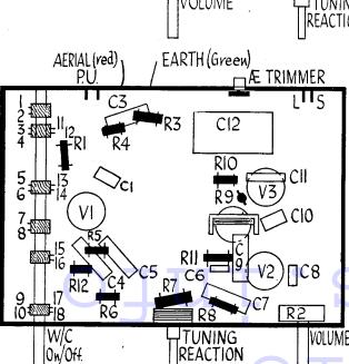
Left, the com-ponent arrangement of the underside of the Cossor 393 chassis. This is simply arranged and should facilitate any service replacement operations.
