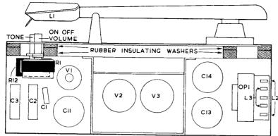
MPLIFIER circuit consists of a high-gain RF pentode VI resistance-capacity coupled to a pentode output valve V2. Output is fed into a 5-in. PM speaker. HT is provided by an indirectly heated half-wave rectifier V3.
