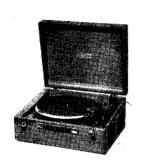
Portable electric gramophone fitted with Collaro induction motor, 12-in. turntable, magnetic pick-up and automatic stop mechanism. Pick-up feeds into two-stage, threevalve amplifier fitted with 5-in. PM speaker. Designed to operate on 50 60 cycle AC mains supplies of 100-125, 200-250 V. Housed in light brown rexine covered carrying case fitted with handle. Manufactured by Collaro Ltd., Barking, Essex.
