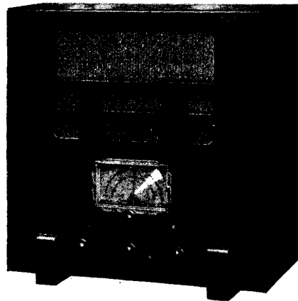
The Alba 501 three-valve plus rectifier receiver made by A. J. Balcombe, Ltd.
