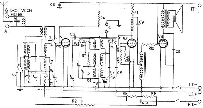
Automatic bias is one of the features of the circuit of the Alba 310 battery three, which gives reception on three wavebands. Iron-cored coils are employed, while an alternative aerial tapping is provided to bring into circuit a Droitwich filter conmosisting of a pre-tuned condenser and coil arrangement.
