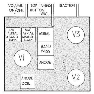
The simple layout of the upper side of the Alba 310 chassis can be seen from the drawing on the left. The chassis can be removed from the cabinet after taking out four bolts and removing the control knobs. If it is necessary to remove the speaker, only four more bolts have to be removed.
