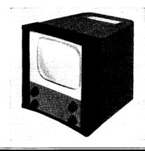
THE receiver employs a superhet circuit, with two RF stages designed to operate on lower sideband of vision carrier. Aerial, RF and oscillator circuits are tunable to any of the five BBC channels. Sound noise and vision interference suppression circuits are fitted, the latter being provided with a continuously variable control for optimum setting. Mains consumption is approximately 120W.
