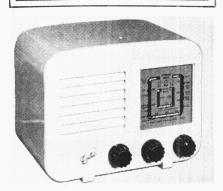
**▼** ANGED permeability variable tuning is a feature of the Dulci MLU5 receiver a model of "midget" construction designed to operate from A.C. or D.C. mains of 200-250 V. The waveband ranges are 187-540 m and 1,200-2,000 m. It is not fitted with a frame aerial, but is intended to be used with a "throw out" flexible aerial. In conformity with midget practice, no provision is made for an earth connection.
