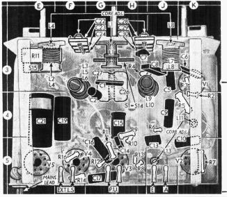
Under - chassis view. The arrow indicating the SI-S14 switch unit shows the direction in which it is viewed in the diagram inset beside the plan view at the top of the page.
