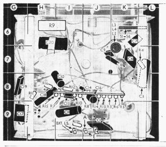
Under-chassis view. Most of the small components are mounted on the group board near the centre of the chassis. The E socket and the Ext-L.S. socket diagonally opposite to it on the rear panel may be transposed.
