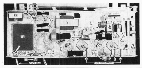
Under-chassis view. The waveband switch unit S1-S10 is indicated here by an arrow which indicates the direction in which it is viewed in the diagram in col. 2 above. R3 and R6 cannot be seen in the actual chassis as they are enclosed in sleeving.
