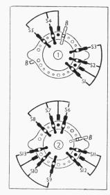
Diagrams of the two waveband switch units, both drawn as seen when viewed from the rear of an inverted chassis. Blank tags are indicated by B. The associated switch table is in the next column.
