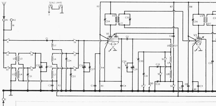
Circuit diagram of the Beethoven A415 3-band A.C. superhet. In the oscillator circuit, C32 and C33 are connected in parallel on while C30 and C31 are in parallel for L.W. On S.W., S12 and S13 close. This results in an unusual sequence of alignment ope and it is important that the instructions overleaf are carried out in the order given. Only the first I.F. transformer has iron-dustriance.
