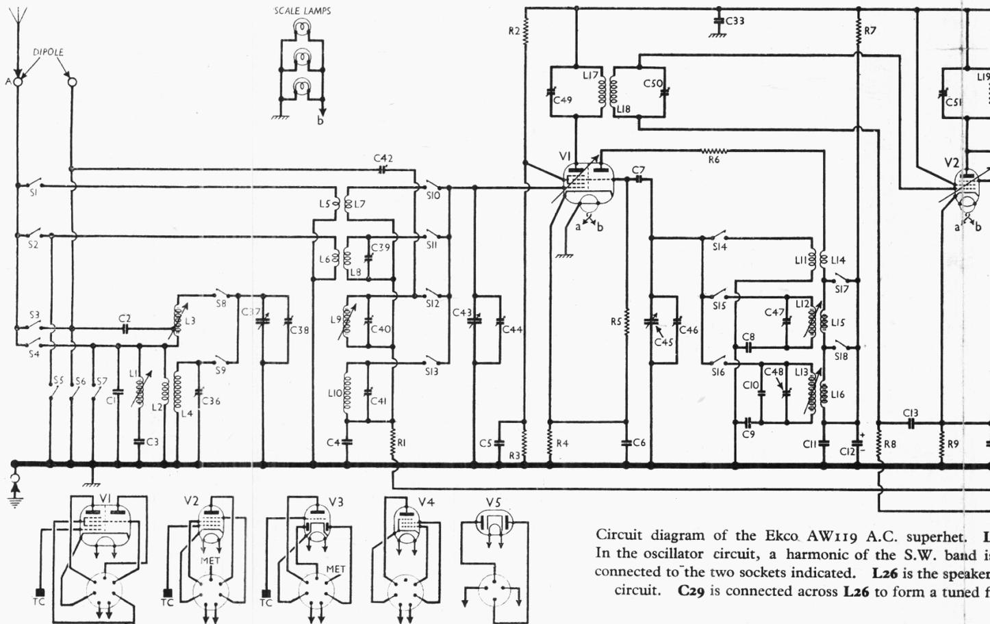
Circuit diagram of the Ekco AW119 A.C. superhet. In the oscillator circuit, a harmonic of the S.W. band is connected to the two sockets indicated. **L26** is the speaker circuit. **C29** is connected across **L26** to form a tuned f
