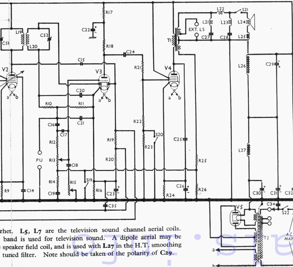
phet. **L5**, **L7** are the television sound channel aerial coils. band is used for television sound. A dipole aerial may be speaker field coil, and is used with **L27** in the H.T. smoothing tuned filter. Note should be taken of the polarity of **C29**.
