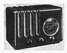
ONSTRUCTED on Midget receiver lines, the Invicta "Piccaninny" model 820 receiver is a 4-valve (plus rectifier) 2-band superhet designed to operate from AC or DC mains of 200-240 V, 40-100 c/s in the case of AC. Provision is made for fitting an additional ballast resistor for operation on 250 V mains, but no provision is made for connecting an earth lead.
