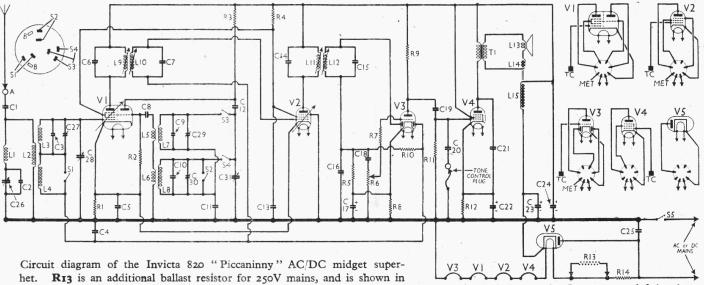
broken lines as it is not normally fitted. When it is used, the shorting link across it is removed. Inset at top left-hand corner is the diagram of the waveband switch unit, drawn as seen from the rear of the underside of the chassis.
