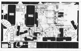
Under - chassis view. The waveband switch unit S1-S4 is indicated here, but it is shown in detail inset in the circuit diagram over-C23 and leaf. C24 be may transposed in some chassis.
