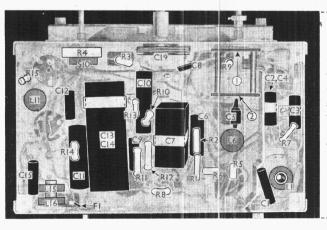
Under-chassis view. The two switch units are indicated, and are numbered to agree with the detailed diagrams of the units above. FI is the mains circuit fuse wire.
