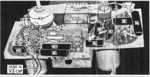
Underside view of receiver chassis. The S1, S2 switch unit is indicated here, and shown in detail in the top left-hand corner of the circuit diagram overleaf. Several components are shown dotted through the mounting panel on the left.
