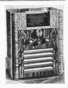
THE Invicta A49 is a 3-valve (plus rectifier) AC superhet covering four wavebands. The SW ranges are 13.5 to 52 m (referred to as SWI in this Service Sheet) and 50 to 200 m (referred to as SW2).
