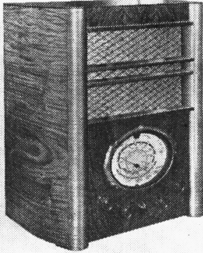
The Burndept 290 table model AC superhet. A push-pull output stage is used.
