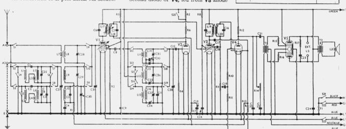
A separate triode oscillator is used in conjunction with a heptode for frequency changing in the Cossor 583 3-band battery superhet. T band-pass input filter has iron-cored coils for the MW band, and the IF transformers are tuned by means of variable iron cores.
