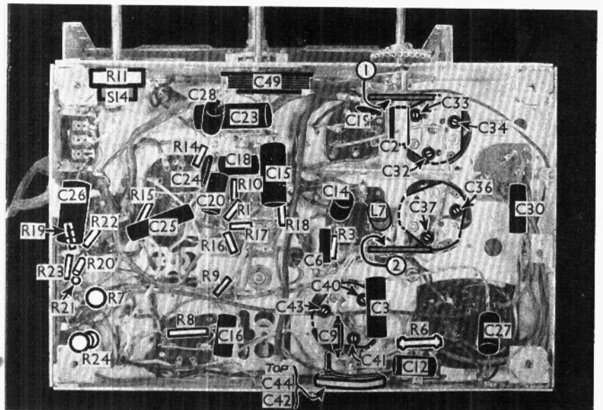
Under-chassis view. The switch units are indicated, and are shown in detail overleaf.
