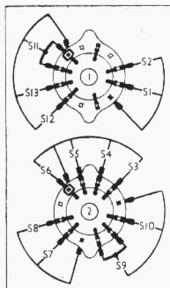
Switch diagrams, looking at the underside of the chassis, in the directions of the arrows in the under-chassis view.
