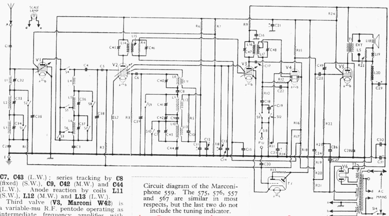
**C7**, **C43** (L.W.); series tracking by **C8** (fixed) (S.W.), **C9**, **C42** (M.W.) and **C44** (L.W.). Anode reaction by coils **L11** (S.W.), **L12** (M.W.) and **L13** (L.W.).
