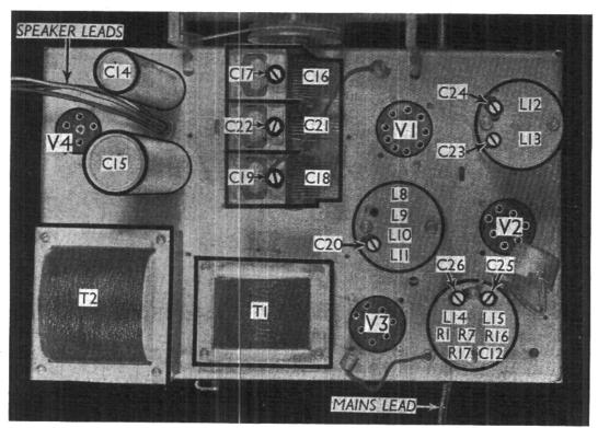
Plan view of the chassis with all trimming condensers clearly shown. The secondI.F.transformer unit contains, apart from its trimmers, five other components (see General Notes). C14 and C15 are H.T. smoothing condensers of the aqueous electrolytic type.
