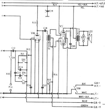
On the left, and on the preceding page is the circuit diagram of the Philco 295. The small letters and arrows assist in tracing across from one section of the diagram to the other.
