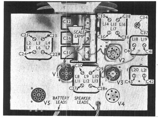
Plan view of the chassis. All trimmers with exception of C21 and C39 are clearly marked.
