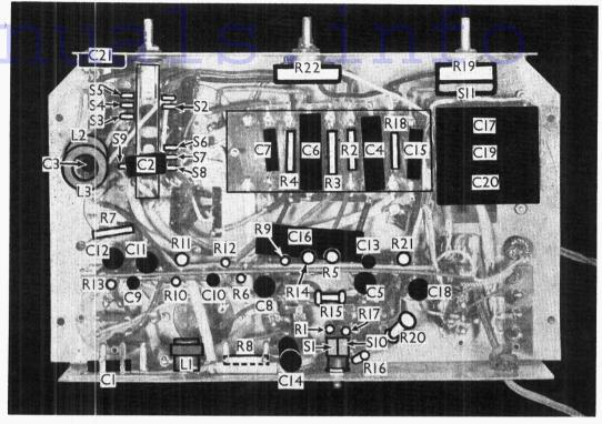
speaker field coil L18 and electrolytic condensers C19, C20.
